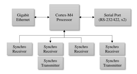
The BBG-7XXX-PCA can support up to four synchro receive channels. Two of the receive channels are factory configurable with synchro transmitters. When ordering, please specify the desired synchro configuration.
