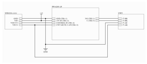
The PW-6295-1P Relay PCB operates on 15 VDC power and a 3-15 VDC relay control voltage. The Relay PCB provides two single-pole single-throw normally open (NO) relay contacts.
